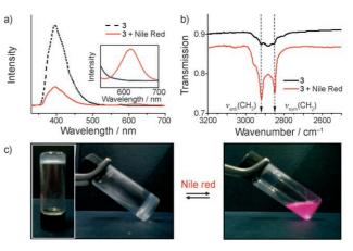
**Figure 4.** a) Emission spectra ( $\lambda_{ex} = 298$  nm) of a solution of **3** ( $2.5 \times 10^{-3}$  M) and a solution of **3** ( $2.5 \times 10^{-3}$  M) and Nile Red (10 mol% relative to **3**). b) FTIR spectra (2500-3200 cm<sup>-1</sup>) of an aqueous solution of **3** (0.1 wt%) and a solution of **3** and Nile Red (0.1 wt%). c) Photographs of the reversible sol–gel phase transition upon addition of Nile Red (2 wt%).
